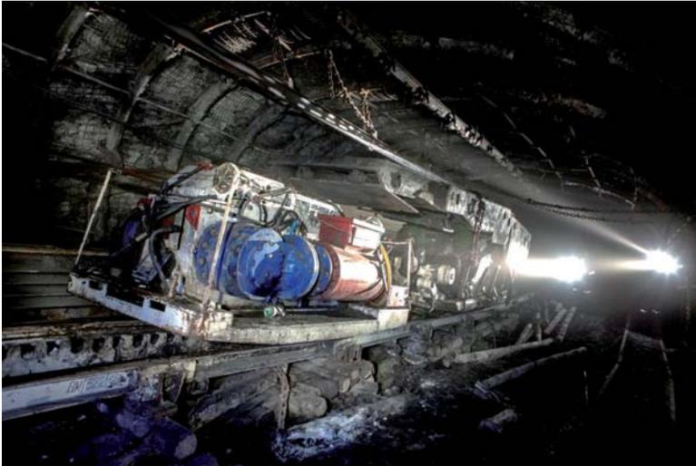
**Figure 4: Diesel floor mounted rack and pinion railway type KSZ-900/110**
