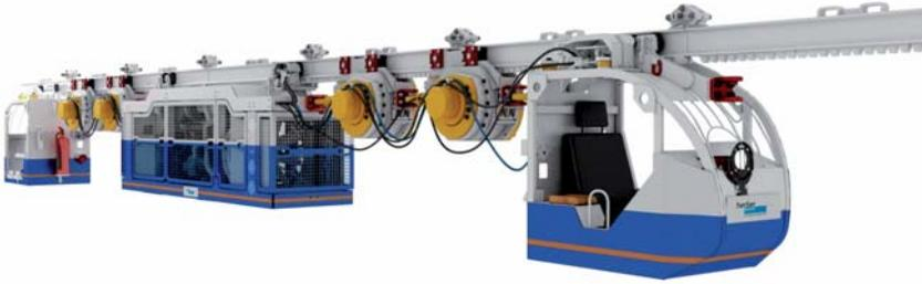
**Figure 3: Diesel toothed suspended railway KP-95**
