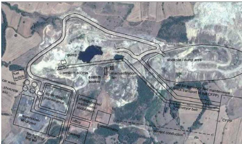
**Figure 8: Surface facilities: detail view**
