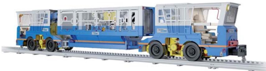
**Figure 1: Diesel toothed locomotive type LZS-150 functioning as the toothed haulage**
